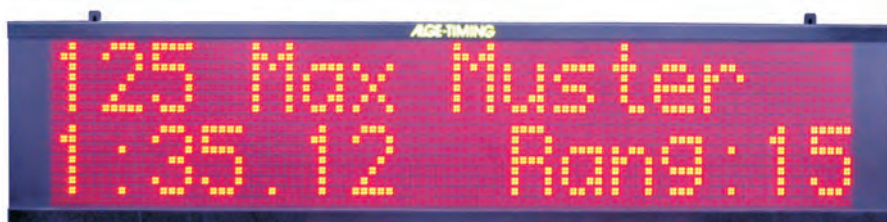
Display board controlled directly from ALGE TdC 8001
