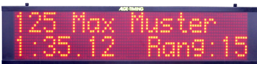
Display board controlled directly from ALGE TdC 8001
