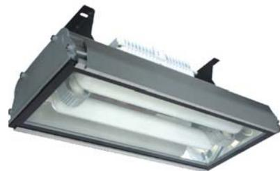
A 400-watt Snow-Bright “down-slope” lamp produces an elongated lighting pattern that can disperse light along the vertical slope contour. Unlike conventional spot lights, the light source is over 2 feet long. Lamps can be canted to accommodate specific slope incline.
