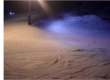
Retrofit project shows sodium on left, metal halide on right, and Snow-Bright center-right. Notice the high contrast without glare on the snow illuminated by Snow-Bright™ lamps
